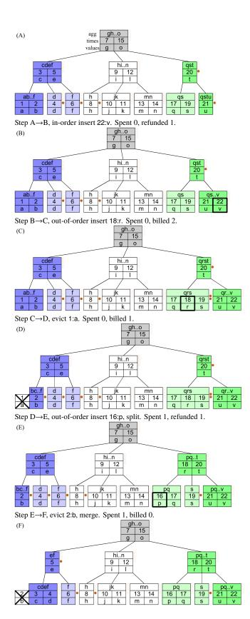
Figure 3: Finger B-tree with aggregates: example.
